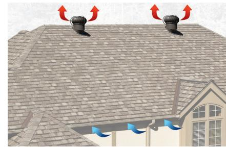
1. Warm, moist air escapes attic through the **Master Flow® Wind Turbines**
